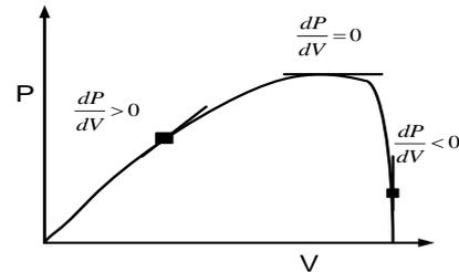
Figure 2. P-V characteristics of solar cell
