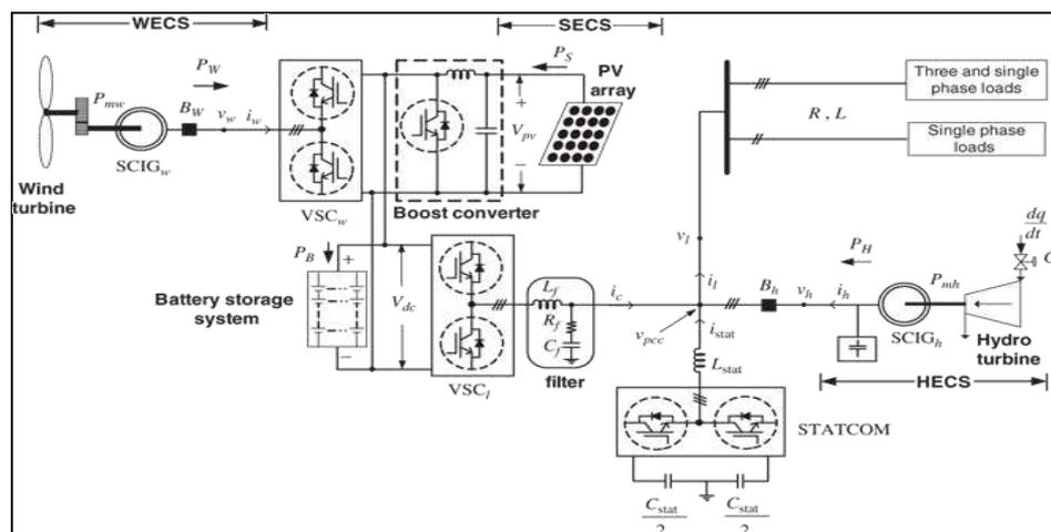
Figure 4. Proposed model for hybrid energy system with solar, wind and small hydro resources
