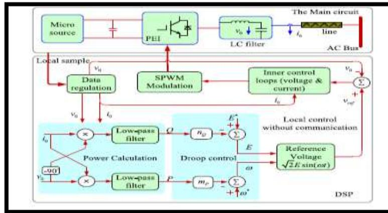
Figure 5. Control structure of conventional  $P/f$  and  $Q/V$  droop control
