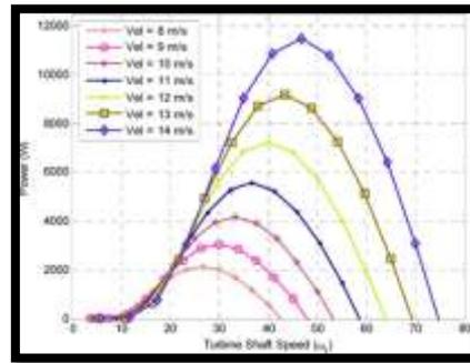
Figure 3. Wind Turbine power curve
