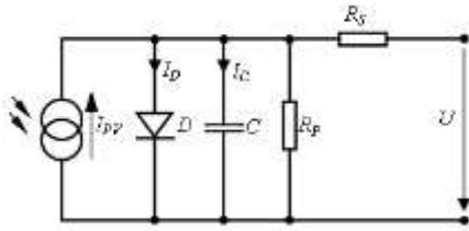
Figure 1. Equivalent circuit diagram of a solar cell
